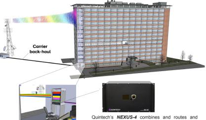
routes multi-carrier's signals to remote antennas
